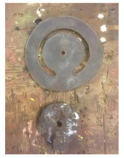
I decided to use modern 43mm plastic waste pipe for the delivery pipe and therefore Araldited a short length of pipe into the end of the pump to make it easy to do the connection. I also bought a standard 43mm non-return valve to fit at the bottom of the pipe to hopefully hold the water in the delivery pipe to make it easy to self-start.
