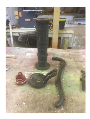
I cleaned up the bore of the pump as well as I could and replaced the bottom flap valve which I made from a piece of 5mm thick leather kindly given to me by our local saddlery company, Penfolds in Cuckfield. After soaking the leather seal in olive oil for two days to soften it, I painted the pump with Hammerite and reassembled it with the new lift valve.
