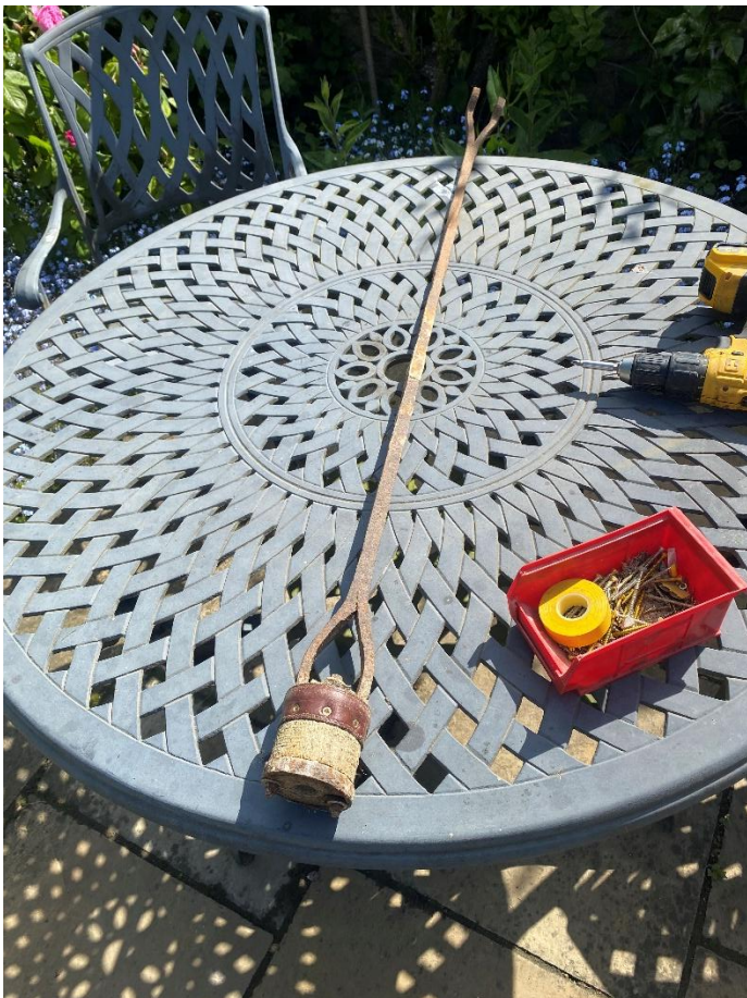
The plunger was refurbished with leather from an old belt
