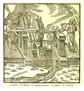
In this woodcut illustration the pump can be seen to involve a series of balls instead of discs, and even earlier versions were described as rag-and-chain pumps.
